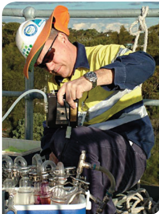
Air quality monitoring during the treatment of contaminated soil for the Car Park Waste Encapsulation Remediation Project
