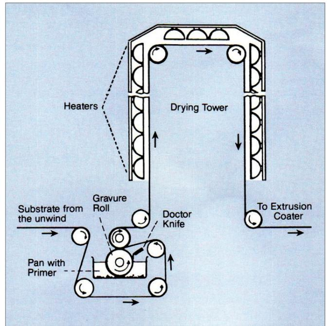
Figure 6: Schematic Drawing of Typical Priming Station
