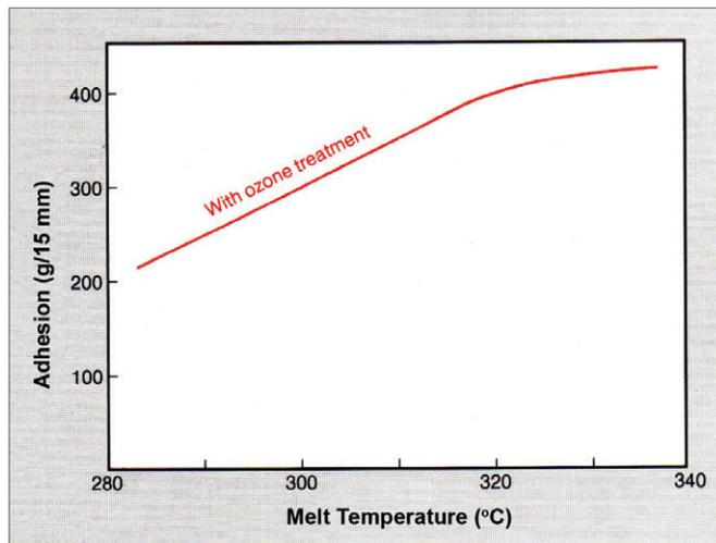
Figure 1: Effect of Melt Temperature and Ozone Treatment on Adhesion of Extrusion-Coated LDPE to Aluminium Foil
