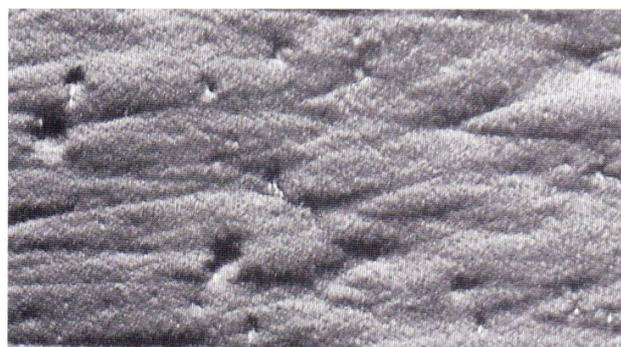
“Orange peel” 100µm  Machine Direction →
