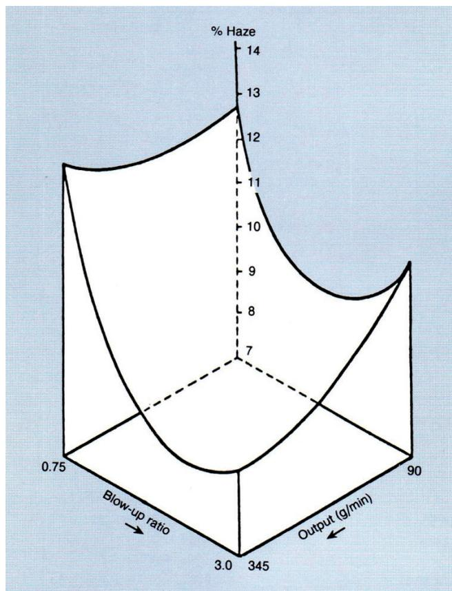
**Figure 5.** Variation of haze with blow-up ratio and output rate for LDPE film of MFI 4.0, density 0.925 g/cm<sup>3</sup>, film thickness 38 µm
