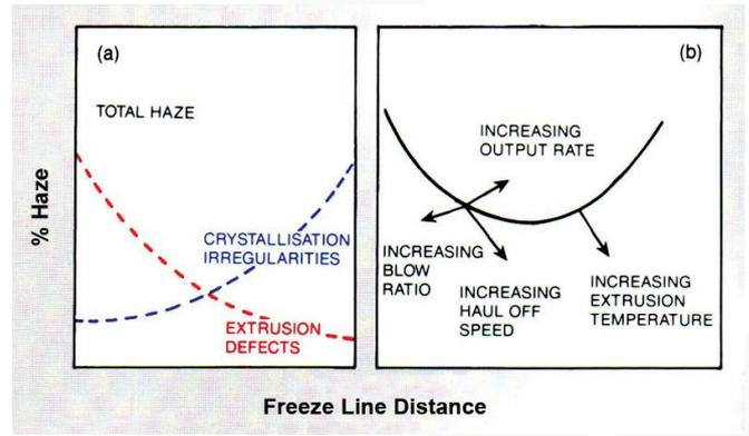
**Figure 2.** Characteristic variation of film haze with freeze line distance for LDPE film
