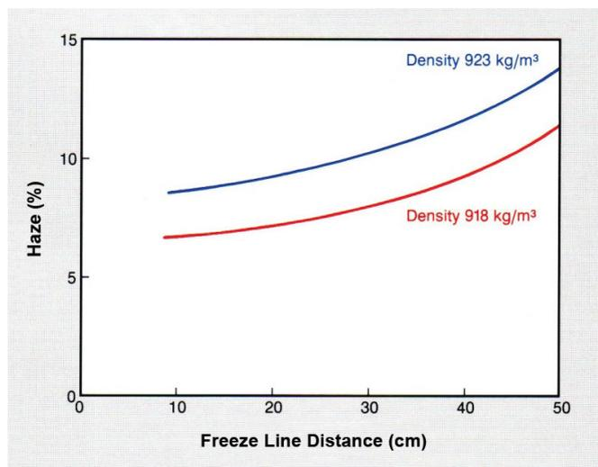
**Figure 4.** Typical variation of haze with freeze line distance for LLDPE film, thickness 40 µm (MFI 0.5)
